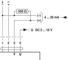
The 500  $\Omega$  resistor converts the 4 ... 20 mA current signal into a voltage signal DC 2 ... 10 V
